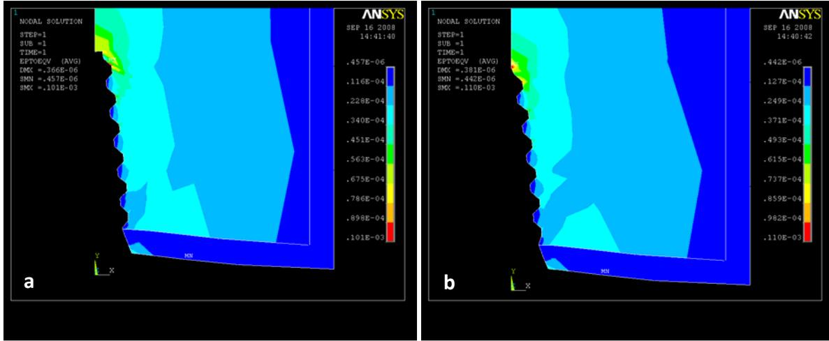
Figure 9. von Mises strain distribution in the conic type 4 with 0.12 gradient from  $.457 \times 10^{-6}$  to  $.101 \times 10^{-3}$  Pa (a) and conic type 5 with 0.16 gradient from  $.442 \times 10^{-6}$  to  $.110 \times 10^{-4}$  Pa; highest max strain is generated in this type (b).
