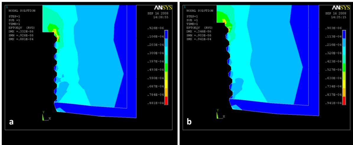
Figure 8. von Mises strain distribution in the cylindrical from  $0.926 \times 10^{-6}$  to  $0.881 \times 10^{-4}$  Pa (a) and conic type 2 with 0.06 gradient from  $0.903 \times 10^{-6}$  to  $941 \times 10^{-4}$  a Pa (b).
